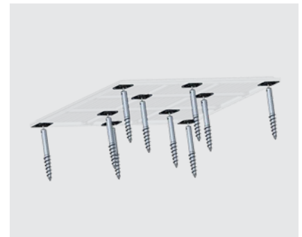
Juno screw foundation 2) The screw foundation contains the ground screws. Support brackets, fixing material and the screw-in aid
